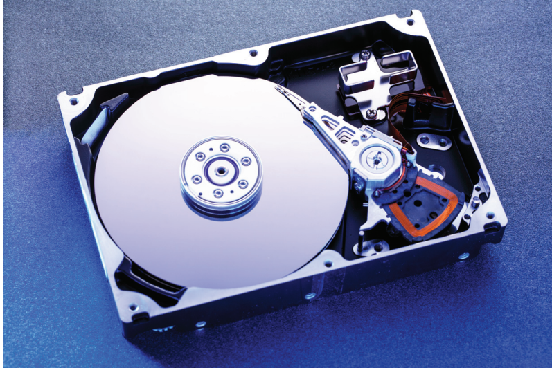
Figure 11.2 A 3.5-inch HDD with cover removed.
