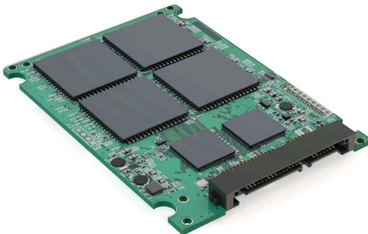
Figure 11.3 A 3.5-inch SSD circuit board.
